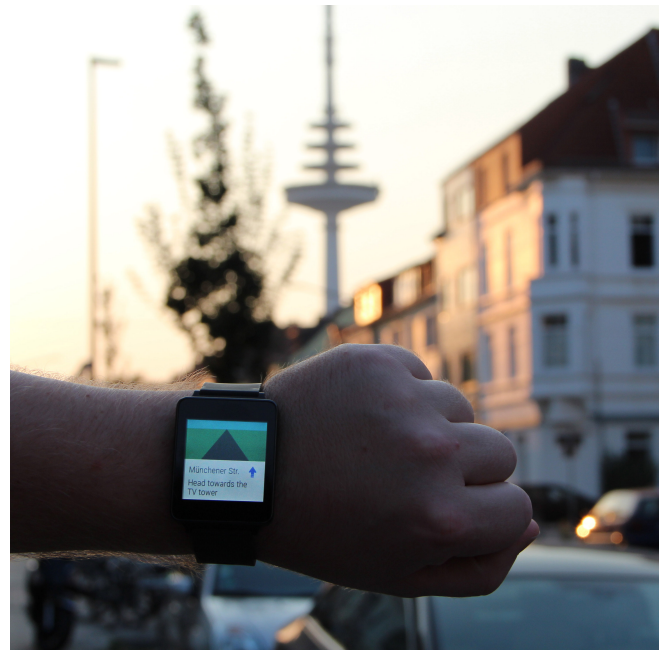
Figure 1: The Pharos navigation approach: Using Google Street View imagery, the visibility of global landmarks (here a municipal TV tower) is determined and then included in the turn-by-turn pedestrian navigation instructions for smartwatches.
