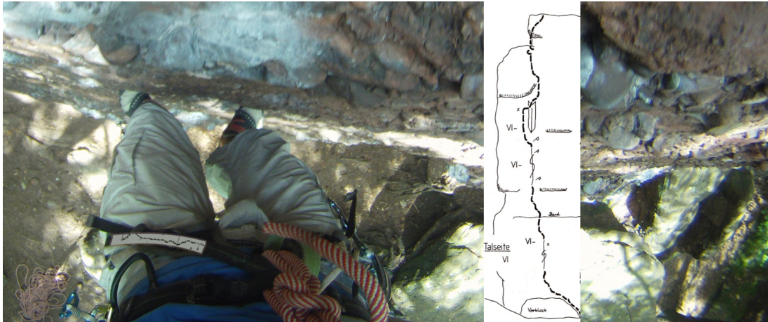
Figure 2: A climbing topo displayed on a StrapMaps attached to a climbing harness (left bottom corner). Compared to Figure 1 no location indicator nor cuts are shown, as no positioning information is available and climbing topos are already linearized (see cutout).
